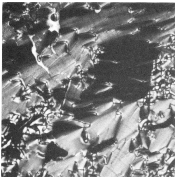
Figure 2. Focal-conic texture of the smectic mesophase of polyester 4 at 212 °C.
