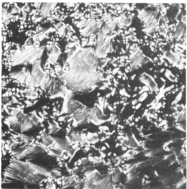
Figure 3. Broken-fan texture of the smectic mesophase of polyester 4 at 188 °C.
